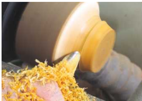
▲ Pic.4 The shape will hopefully end up as an ogee (a flattened S); always go really slow as you get to the centre because the wood is going much slower at this point
